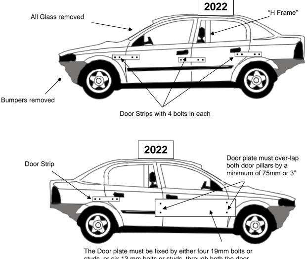
studs, or six 13 mm bolts or studs, through both the door pillars. No slotted holes allowed
